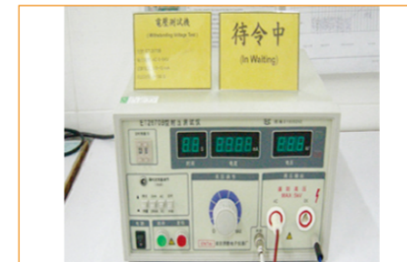
Dielectric Withstanding Voltage
