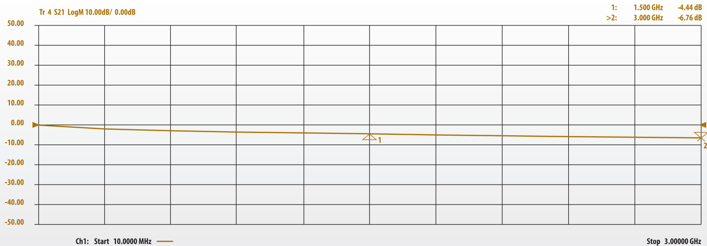
Figure 1b: V73263 Loss at 20 ft
