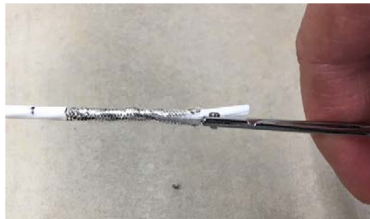
Use a small scissors to cut shield lengthwise
