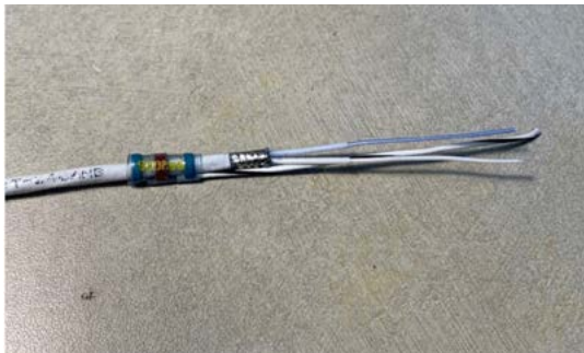
*Ready to heat your solder over shield
