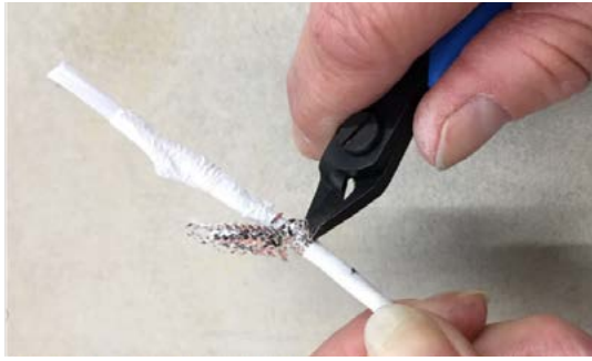
Cut shield off completely
