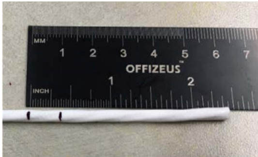
Mark cable at desired strip length for a solder sleeve
