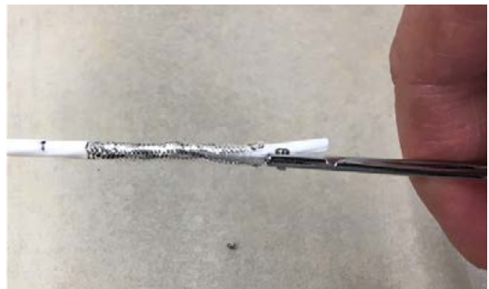
Use a small scissors to cut shield lengthwise
