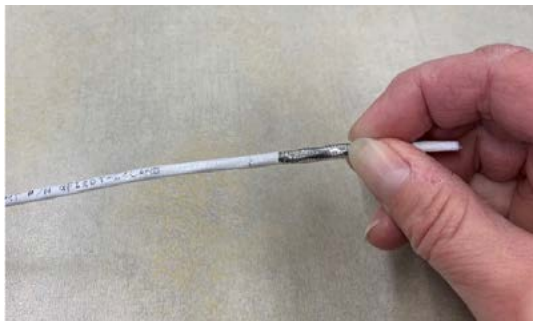
Push shield back to bunch it up
