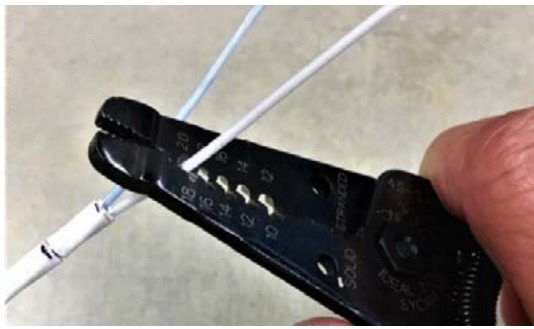
Remove outer insulators. Use a 20 AWG stripper
