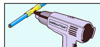
Apply heat to the GREMSEAL® using the air gun.
